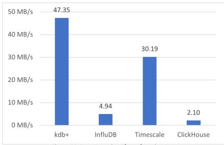
Figure 11: Data Ingestion Throughput in MB/s
